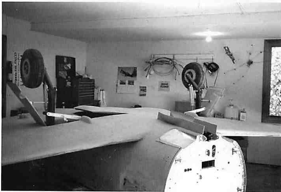
Duane Root's ceiling was too low for his Falco, so he cut a hole in the floor.
