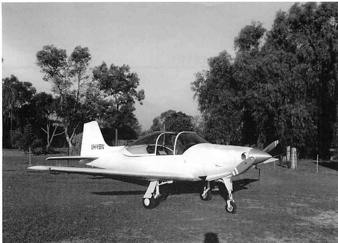
Ian's Falco has a 180 hp IO-360 engine and weighs 1,294 lbs in primer paint only.
