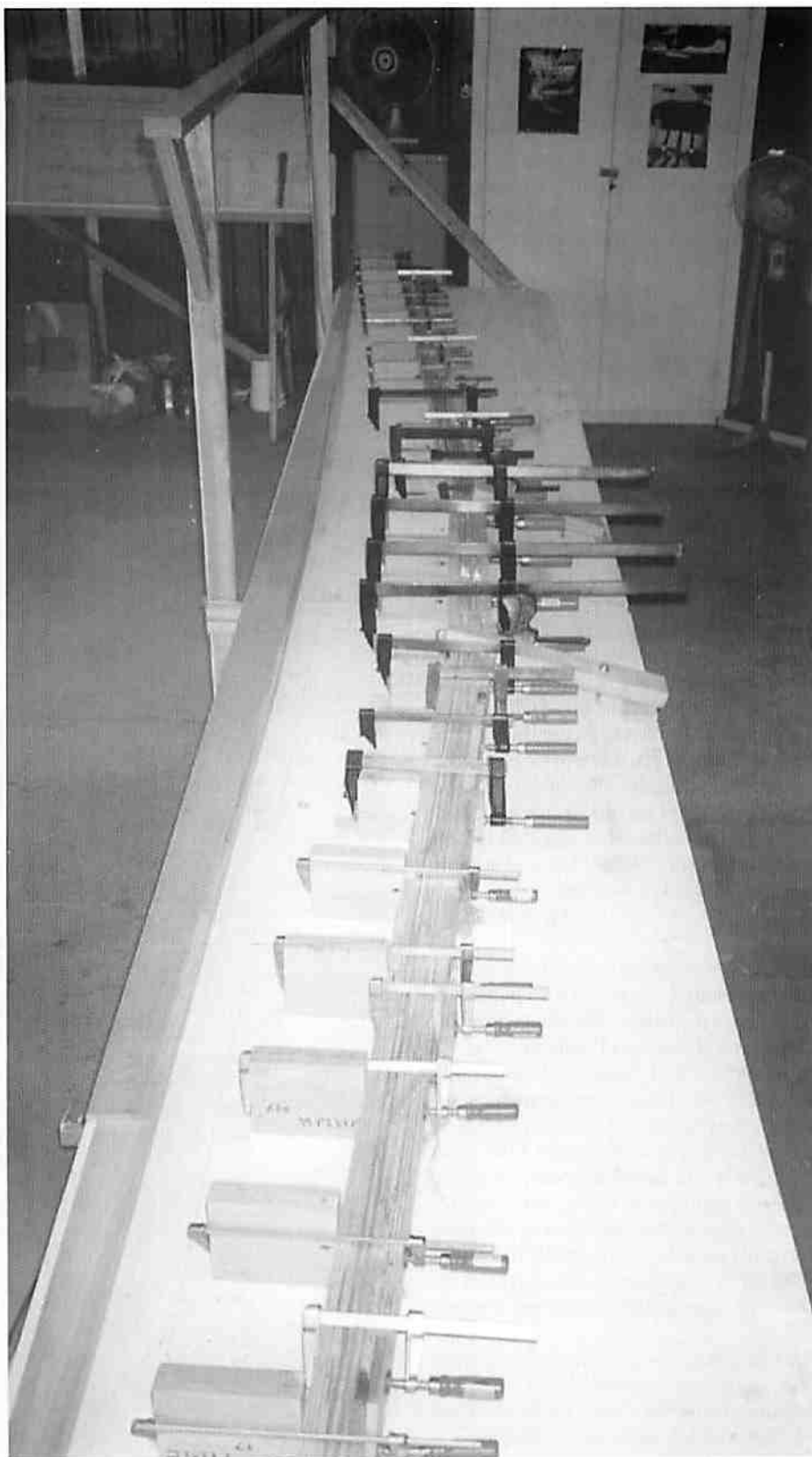
Neil Aitkenhead's main wing spar laminations being glued on the jig table.
