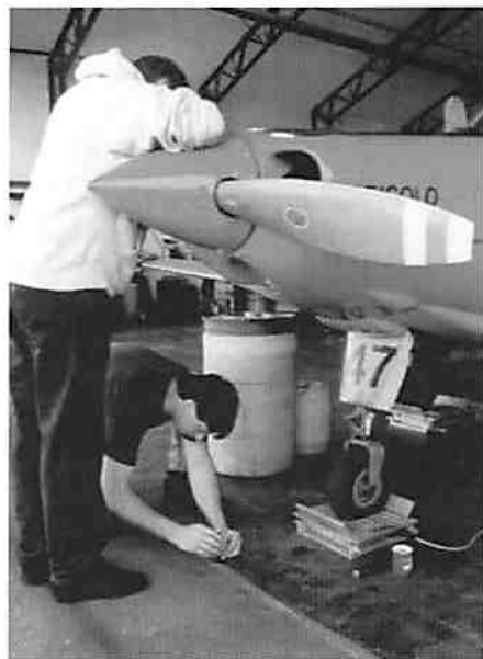
Above: Hanging a plumb line to locate the datum.
