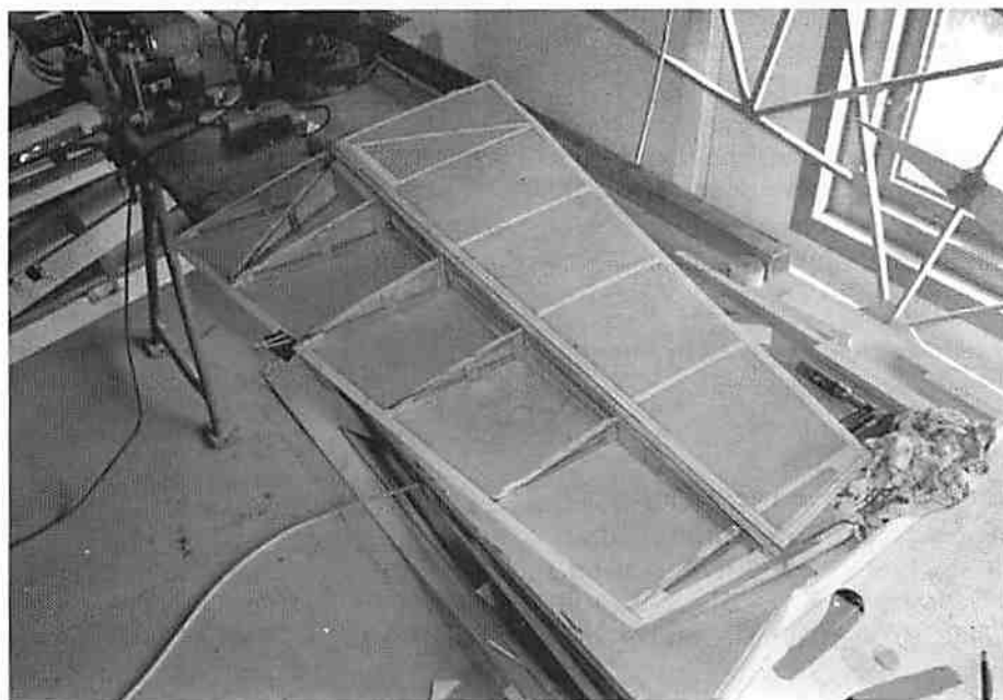
International spruce. Top: Richard Marks' wing takes shape in England. Above: Fedrigo Gilbert's rudder ready for closing in France.
