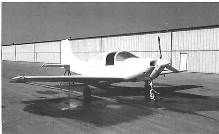
Above center: Willard Hofler's Falco lacks only the cowling, prop and interior. Bottom: Butch Harbold's Sequoia 300 nears completion but is very seriously tail-heavy and will require a ten-inch movement of the engine to get it in balance.
