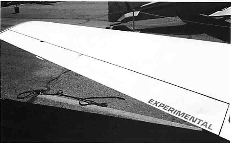
Rex Hume: "After considerable discussion at the West Coast Falco Fly-In that cutouts and access doors are not necessary on the top of the wing—keep it clean."
