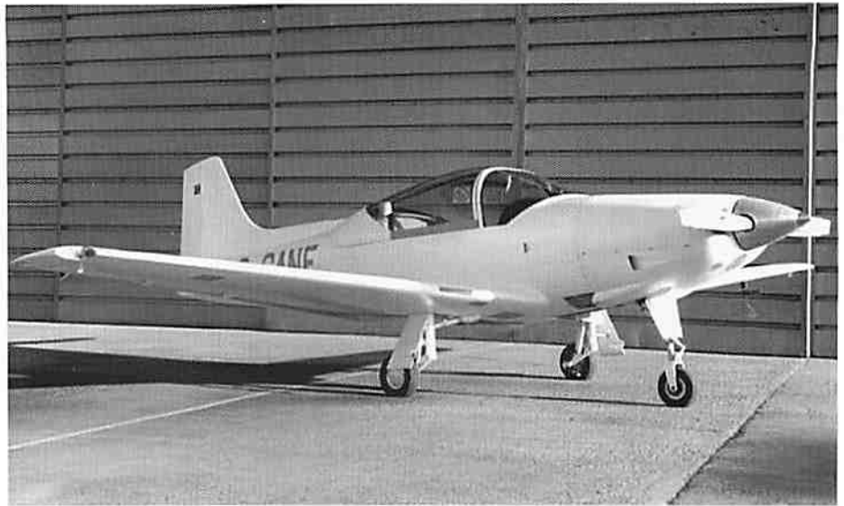
The raised device in the back of the canopy is the GPS antenna.
