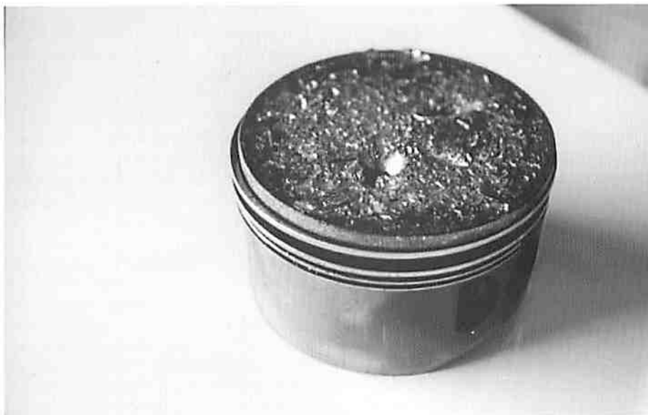
Top: Blake Jessen and his lil' ol' C-5A. Center: The Corporate Disgrace weeps oil. Bottom: What happens when an exhaust valve is digested.
